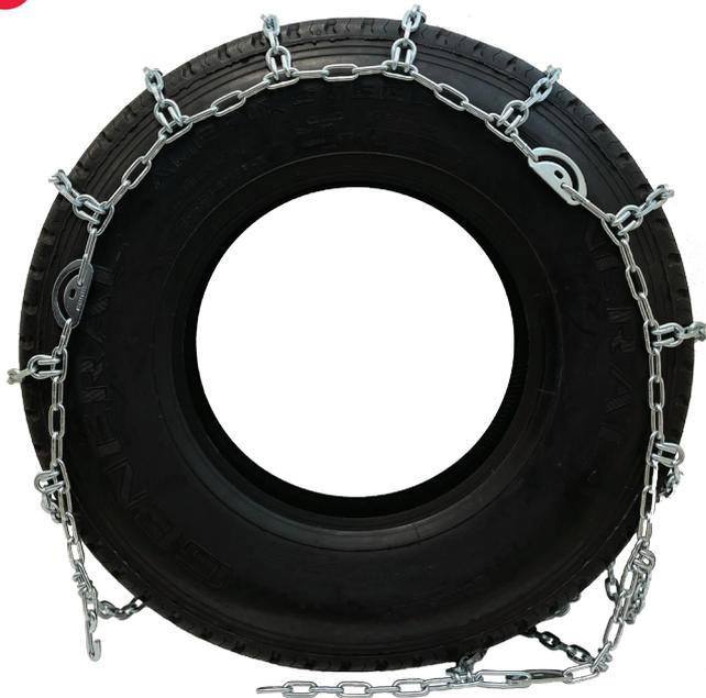
Lay the chains out on the ground with the cross chain hooks facing up, make sure there are no twists in the chain. Grab the middle of the chain and lay them evenly on top of the tire with the cams on the outside of the tire. Cross chain hooks should be facing away from the tire (see picture). Tuck the end of the chains in the rear of the tire and rollback about 2 feet if space allows.
