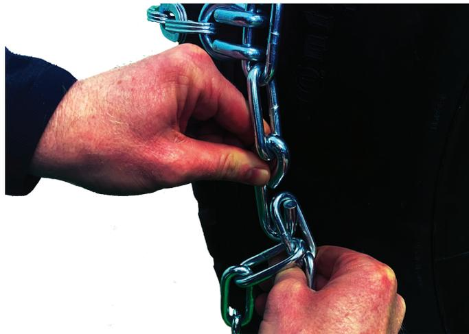
Start by hooking the speed hook on the inside of the tire, and then fasten the hook on the outside of the tire. Try and have them even or close to the same link on the inside as the outside, so one side chain isn't pulling more than the other. Try to get the inside and outside side chain as tight as possible.
