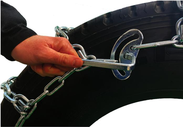
If your chain has cams, use the cam tool in the bag to turn the cams counter-clockwise, start with the lowest cam on the tire. You want the chain to be tight enough to get your knuckles under a cross chain and have pressure. You do not have to turn all the cams in some situations if the chain is tight. Do not over tighten the chain, this can lead to tire damage.
