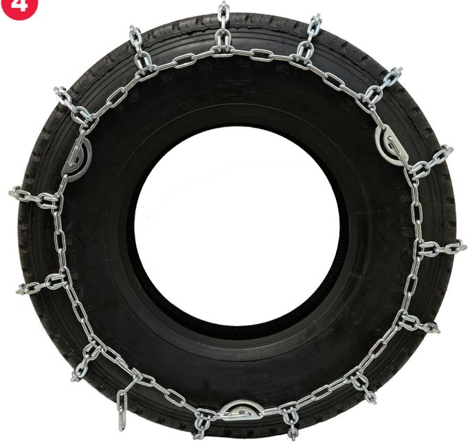
If you are in a safe situation, drive 150-300 feet and let the chain center on the tire. Check for tightness and make sure the chain is centered like the picture shows. Often times you can close the last cam at this point to get a good fit, or you might need to undo the cams and get one more link tighter on the outside speed hook. Then re-tighten cams for proper fitment. Multi-arm adjuster recommended.
